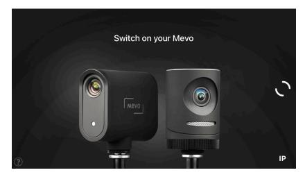
Once you have setup the camera securely attached to the tripod, locate the power button on the backside of the camera and hold down until you hear the initiation chime.
